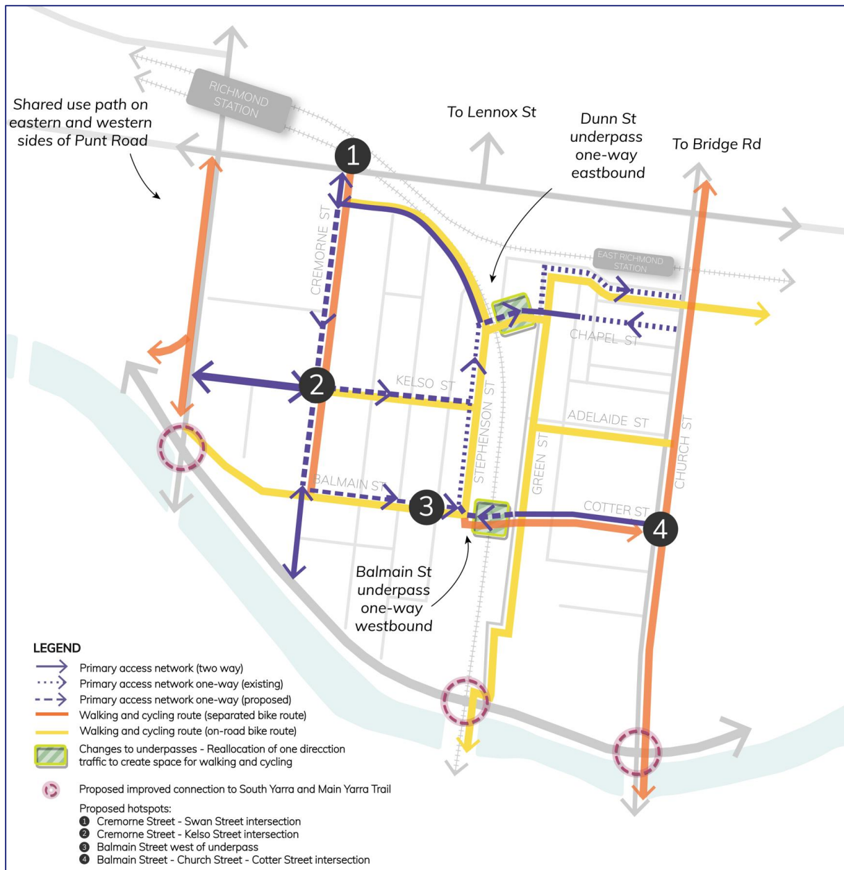
Figure 21: Proposed Future Movement Framework (Source: Proposed future movement network provided to Traffic Group by Council)
