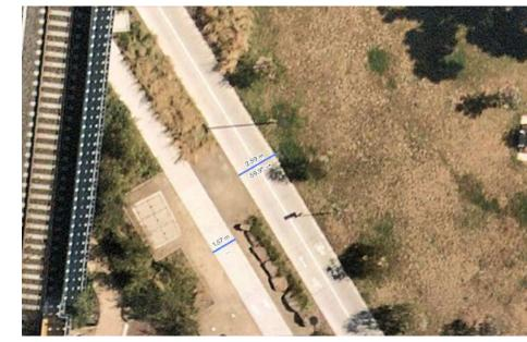
Mernda bike path uses a 3.0m wide bike path alongside a 1.8m pedestrian path
