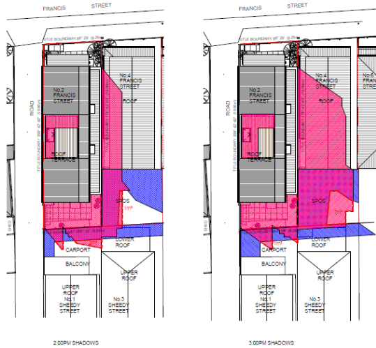
Figure 5: Advertised shadow diagrams at 2pm (left) and 3pm (right) which do not take into account 3D built form and roof form and inaccurately depict shadowing to the roof at No.4 Francis Street
