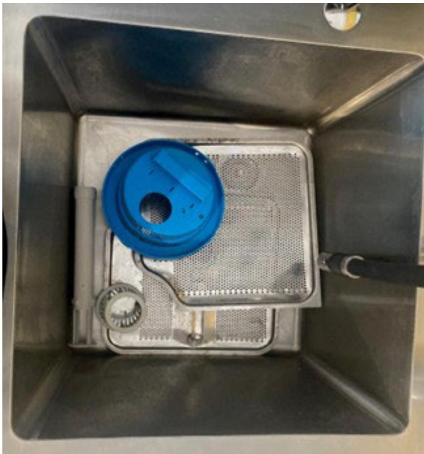
3. Select then “m” button to drain. Light will flash while draining. Once light has stopped flashing, drain cycle is complete. This takes approximately 5 mins.
