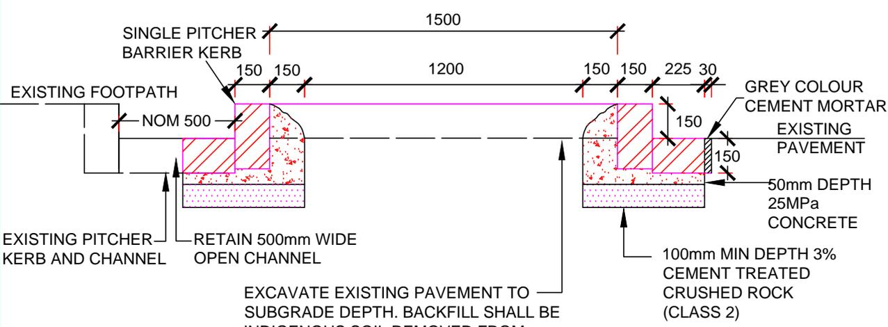
EXCAVATE EXISTING PAVEMENT TO SUBGRADE DEPTH. BACKFILL SHALL BE INDIGENOUS SOIL REMOVED FROM HOLE AND IS TO BE FREE FROM ANY FOREIGN MATERIAL. WHERE EXTRA BACKFILL SOIL IS REQUIRED, THE SOIL SHALL BE CONSISTENT WITH THE INDIGENOUS SOIL. THE FINISHED SURFACE SHOULD BE 100mm BELOW THE TOP OF NEW KERB. TOP WITH 100mm, 12-20mm PINE BARK MULCH.
