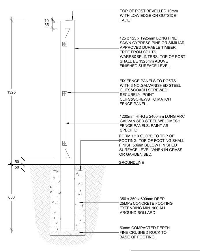
NOTE: ALL METAL COMPONENTS SHALL BE HOT DIP GALVANISED PRIOR TO PAINTING
