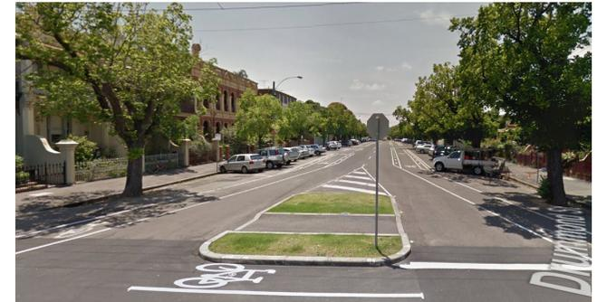
DBYD search shows there are gas lines and NBN near the kerb (service proving needed to confirm proximity to kerb)
