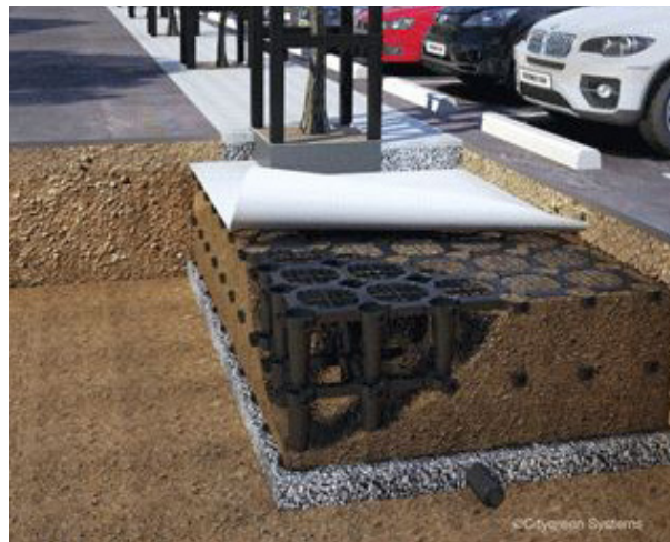
5. Proprietary structural soil systems (e.g. Citygreen Stratavault)
