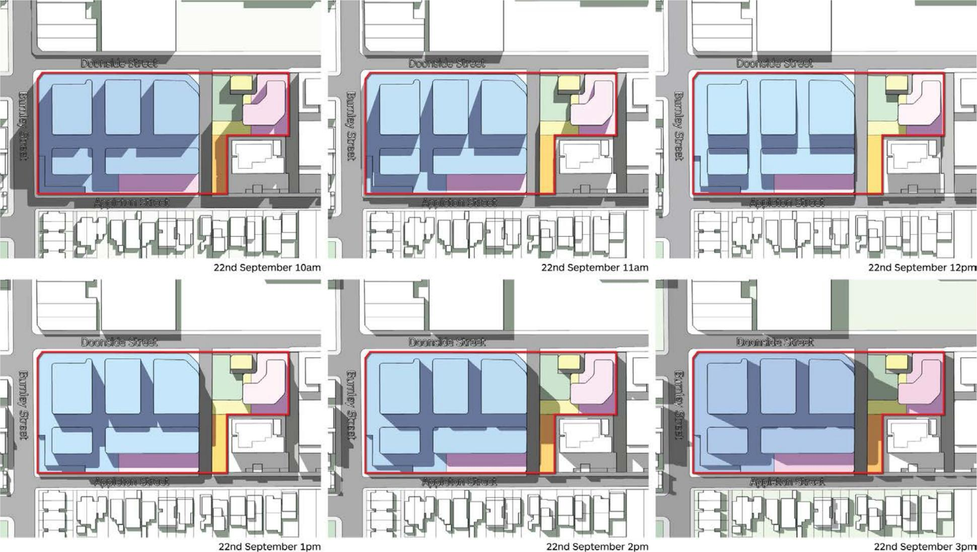
Figure E1 - Shadow Diagrams of The Indicative Framework Plan
