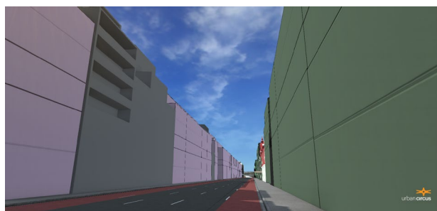
Figure 8.7: East of rail, maximum 18m street wall just avoids shadows on southern footpath
