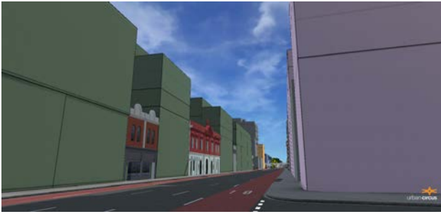
Fig.2.6 East of rail, 18m street wall and reduced to one storey more than heritage facades
