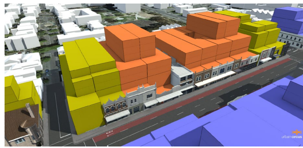
Figure 8.21: Effect on smaller sites of no side setbacks or 4.5m side setbacks above five storeys
