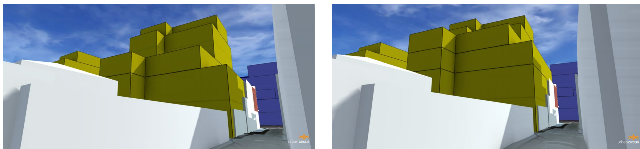
Figure 8.14: Rear interface heights of 11m and 14m to GRZ, with 45° setback above
