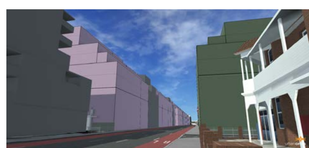
Fig.3.9 Modelled 3m and 45° setbacks above 18m street wall – upper and street views
