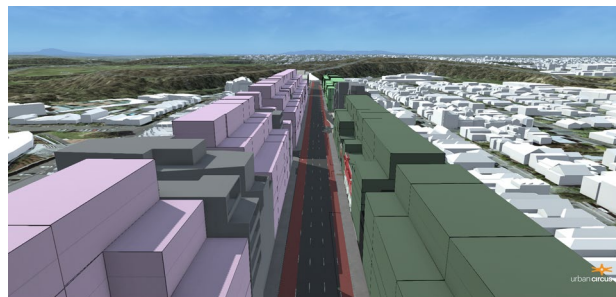
Figure 8.7: East of rail, maximum 18m street wall just avoids shadows on southern footpath
