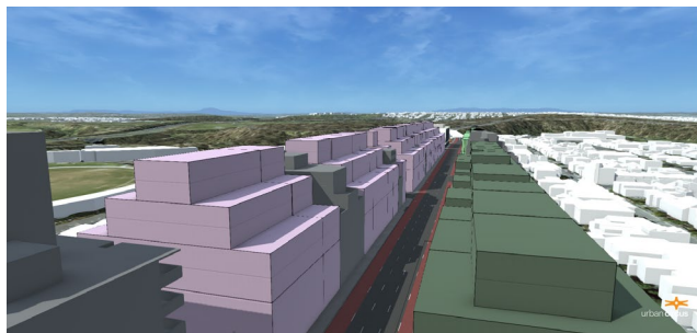
Figure 8.11: Modelled 6m and 45° setbacks above 18m street wall – upper and street views
