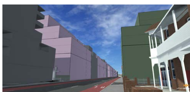
Fig.3.8 Modelled 6m and 45° setbacks above 18m street wall – upper and street views
