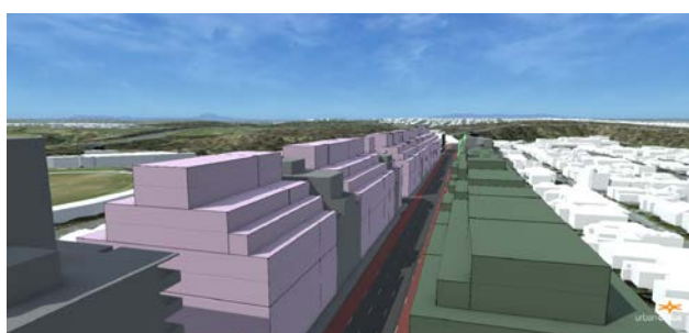
Fig.3.9 Modelled 3m and 45° setbacks above 18m street wall – upper and street views
