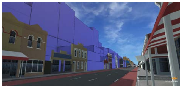
Fig.3.4 No 45^\circ setback allows shadowing
