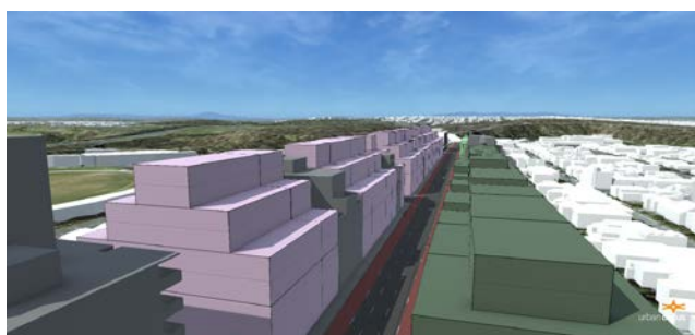
Fig.3.8 Modelled 6m and 45° setbacks above 18m street wall – upper and street views
