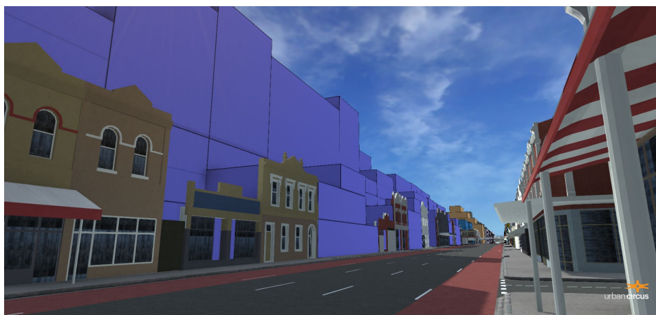
Figure 8.9: Straight-up from 6m setback and continuous stepping at 45°
