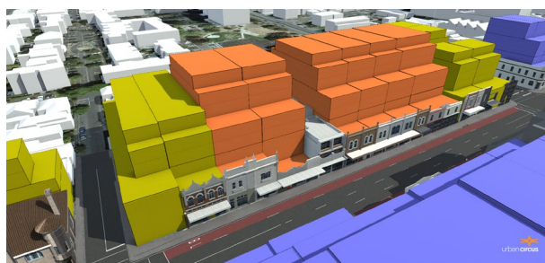
Figure 8.21: Effect on smaller sites of no side setbacks or 4.5m side setbacks above five storeys
