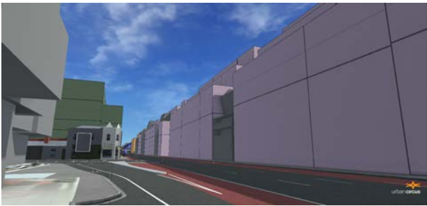
Fig.2.7 East of rail, 18m street wall just avoids shadows on southern footpath
