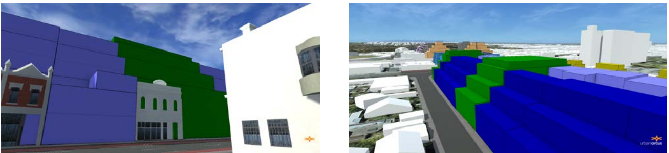
Fig.6.2 Overall height up to 28m (deeper site in green) – street and upper views
