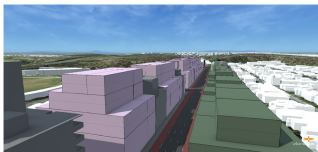
Figure 8.12: Modelled 6m setbacks straight up above 18m street wall – upper and street views
