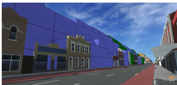
Figure 8.8: 45° setback above theoretical 11m street wall and directly above the heritage parapets
