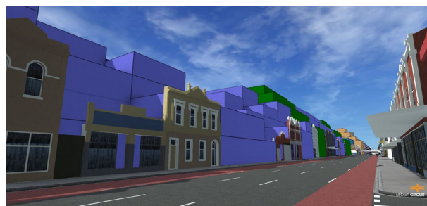
Figure 8.8: 45° setback above theoretical 11m street wall and directly above the heritage parapets
