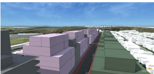
Fig.3.10 Modelled 6m setbacks straight up above 18m street wall – upper and street views
