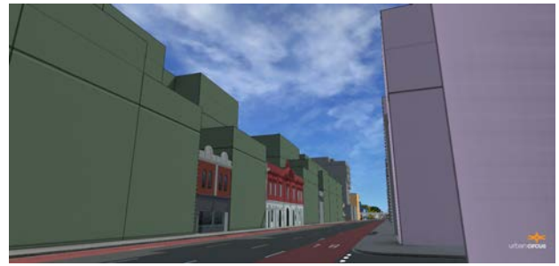
Fig.2.6 East of rail, 18m street wall and reduced to one storey more than heritage facades
