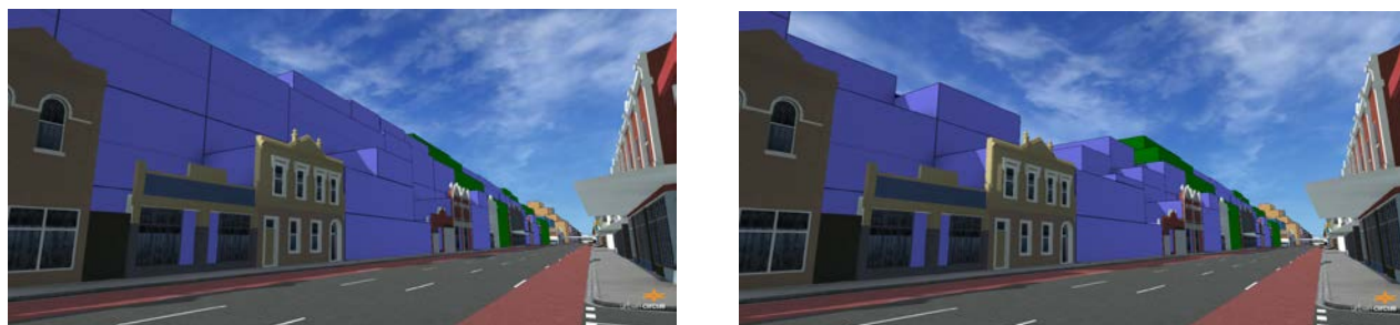
Fig.3.3 45^\circ setback above theoretical 11m street wall and directly above heritage parapets
