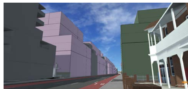
Fig.3.10 Modelled 6m setbacks straight up above 18m street wall – upper and street views
