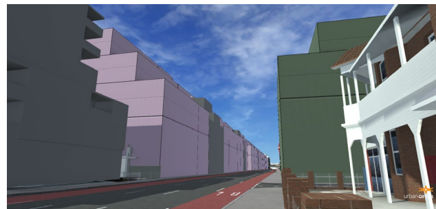
Figure 8.11: Modelled 6m and 45° setbacks above 18m street wall – upper and street views
