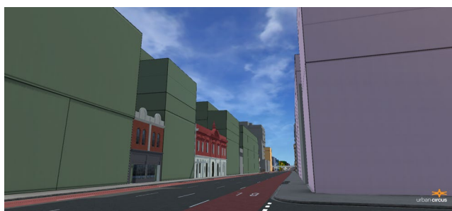
Figure 8.6: East of rail, 18m street wall and reduced to one storey more than heritage building(s)
