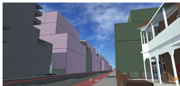
Figure 8.12: Modelled 6m setbacks straight up above 18m street wall – upper and street views
