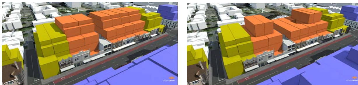
Fig.9.2 Effect on smaller sites of no side setbacks or 4.5m side setbacks above five storeys
