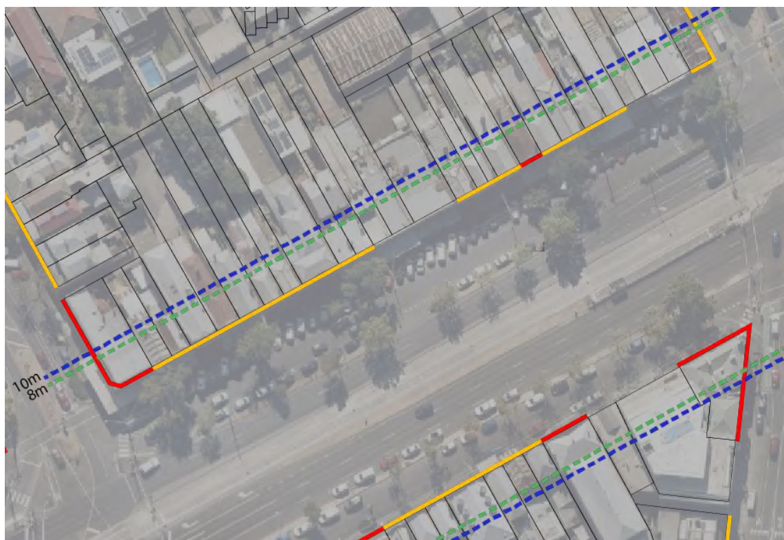
Fig.7.17- Sample Precinct 4 roof plan with 8m (green) and 10m (blue) setbacks
