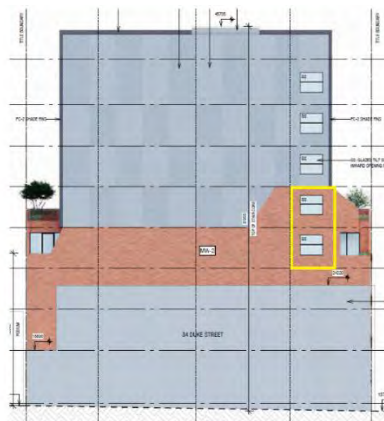
Figure 16. North elevation identifying boundary windows.
