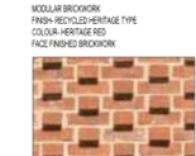
[BMT] MODULAR BRICKWORK FINISH-RECYCLED HERITAGE TYPE COLOUR-HERITAGE RED FEATURE EXPRESSED BRICKWORK
