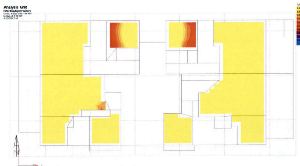
Figure 3: Level 1 Apartments Daylight Modelling Results (Optimised)
