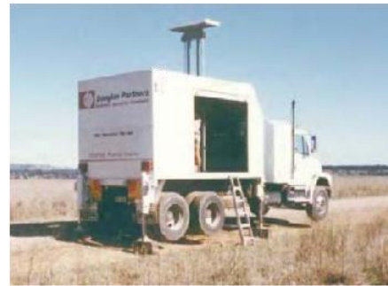
Figure 2: Purpose built CPT rig
