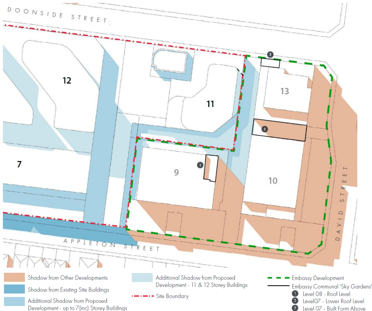
Figure 3 – September Equinox Shadow at 2pm – Common area analysis (Tract Consulting)
