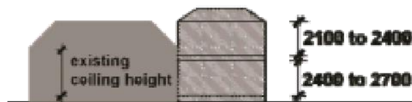
Figure 9 Using ceiling heights as a guide to height of two storey additions
