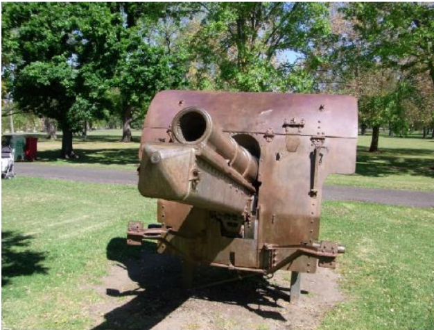
The Collingwood Howitzer prior to its removal from the gardens showing the relatively remarkable condition of the steel fabric, which appears to be protected by a wax coating
