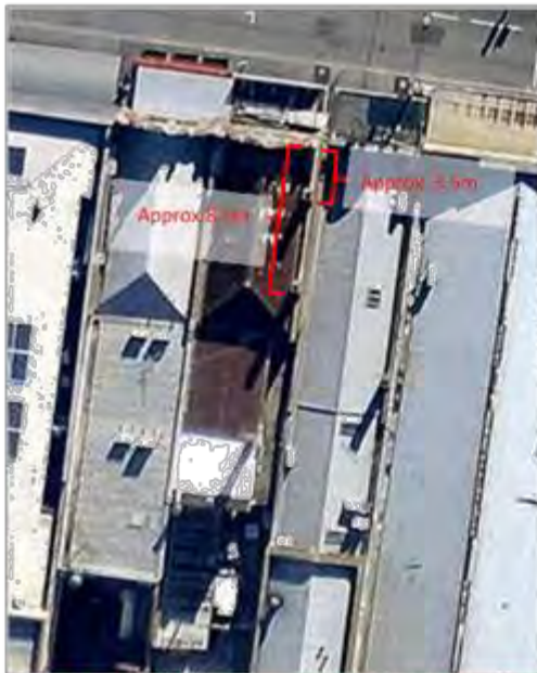
Figure 13. Roof plan (©nearmap, 9 Aug 2017) showing the typical location of chimneys at the centre of each of the front two rooms on the party wall i.e. approx. 3.5m and 8.5m back from the front façade
