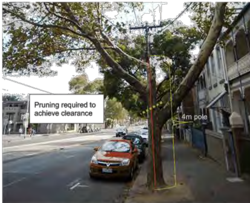
Figure 2: Pruning required to achieve 4.8m over the road. This tree will not remain viable (Tree 13).
