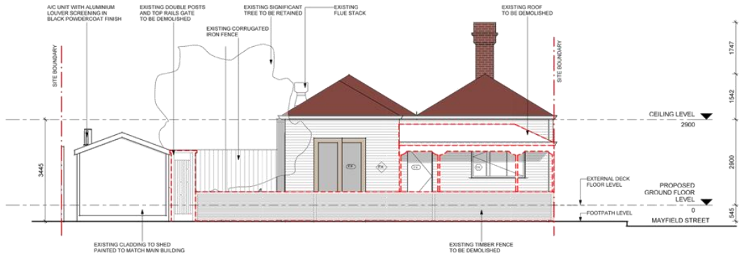
2 EXISTING & DEMOLITION SOUTH ELEVATION (MURRAY STREET) A-0.03' 1:50
