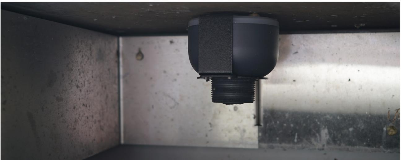
28 A sensor fitted inside one of 600 public bins, to provide real-time data on waste levels.
