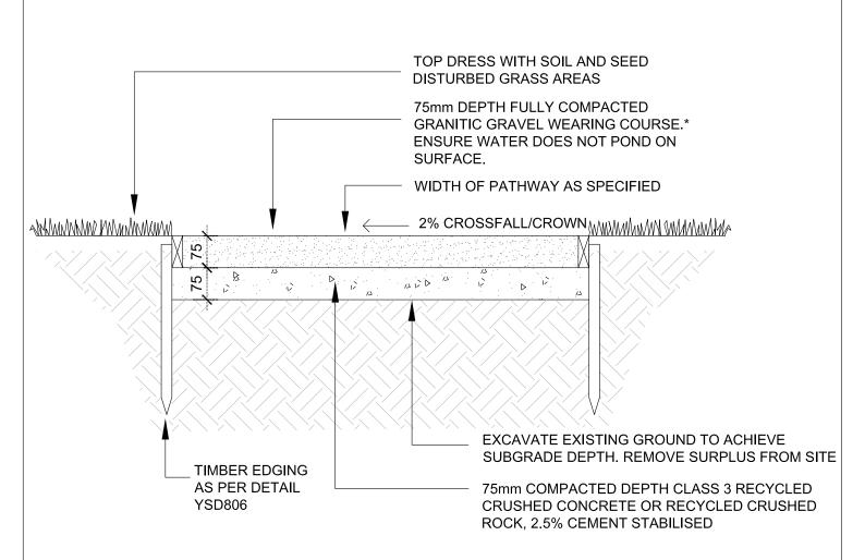
\*NOTE: GRANITIC SAND AS SUPPLIEDBY BURDETT'S SOIL AND GRAVEL SUPPLIES OR EVETTS SOIL AND SAND (or similar as approved by CoY supervisor). FINE GRAINED, YELLOW/BROWN, LOW PLASTICITY, WITH MAX. SILT CONTENT OF 6% BY VOLUME AS PER AS 1141-33.
