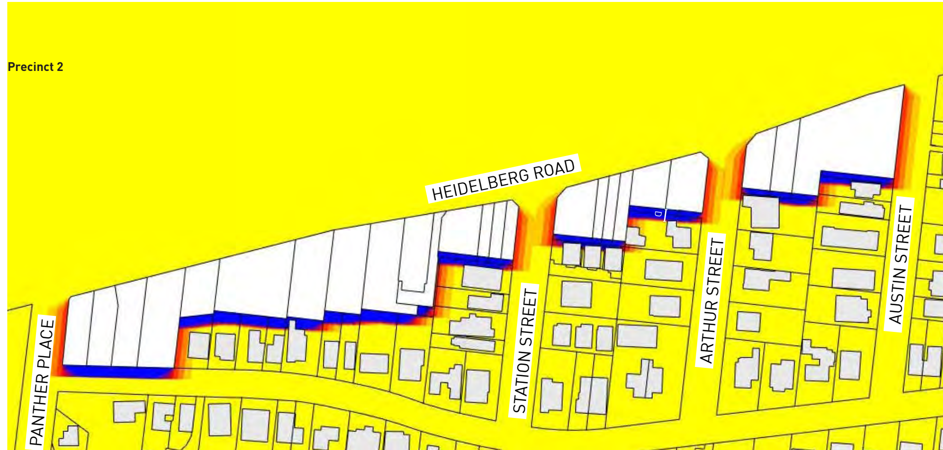
Figure 171. Sunlight hours analysis against Clause 54/55 requirements - 8 metres rear boundary wall height (D=7.7 metres)
