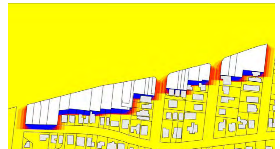
Figure 170. 12 metres rear street wall height (D=11.6 metres)
