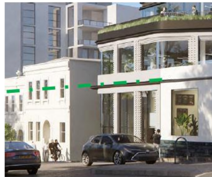
Figure 23: Excerpt from photomontage (Urban Context Report) highlighting different alignment of expressed canopy line relative to neighbouring building (middle of that building's windows).
