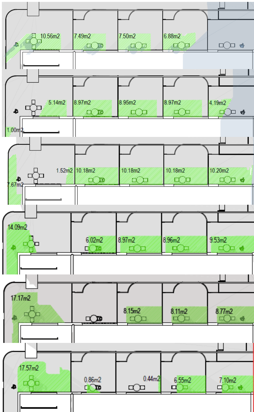
Figure 16: Retained solar access (shown in green, with 9am at top and 3pm at bottom) to the ground floor areas of SPOS of dwellings TH06 – TH10 (Applicant submission, December 2020)
