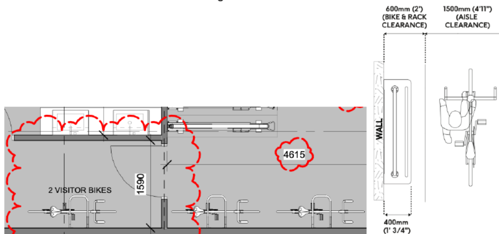
3 Halo racks do not meet the product specification clearance requirements
