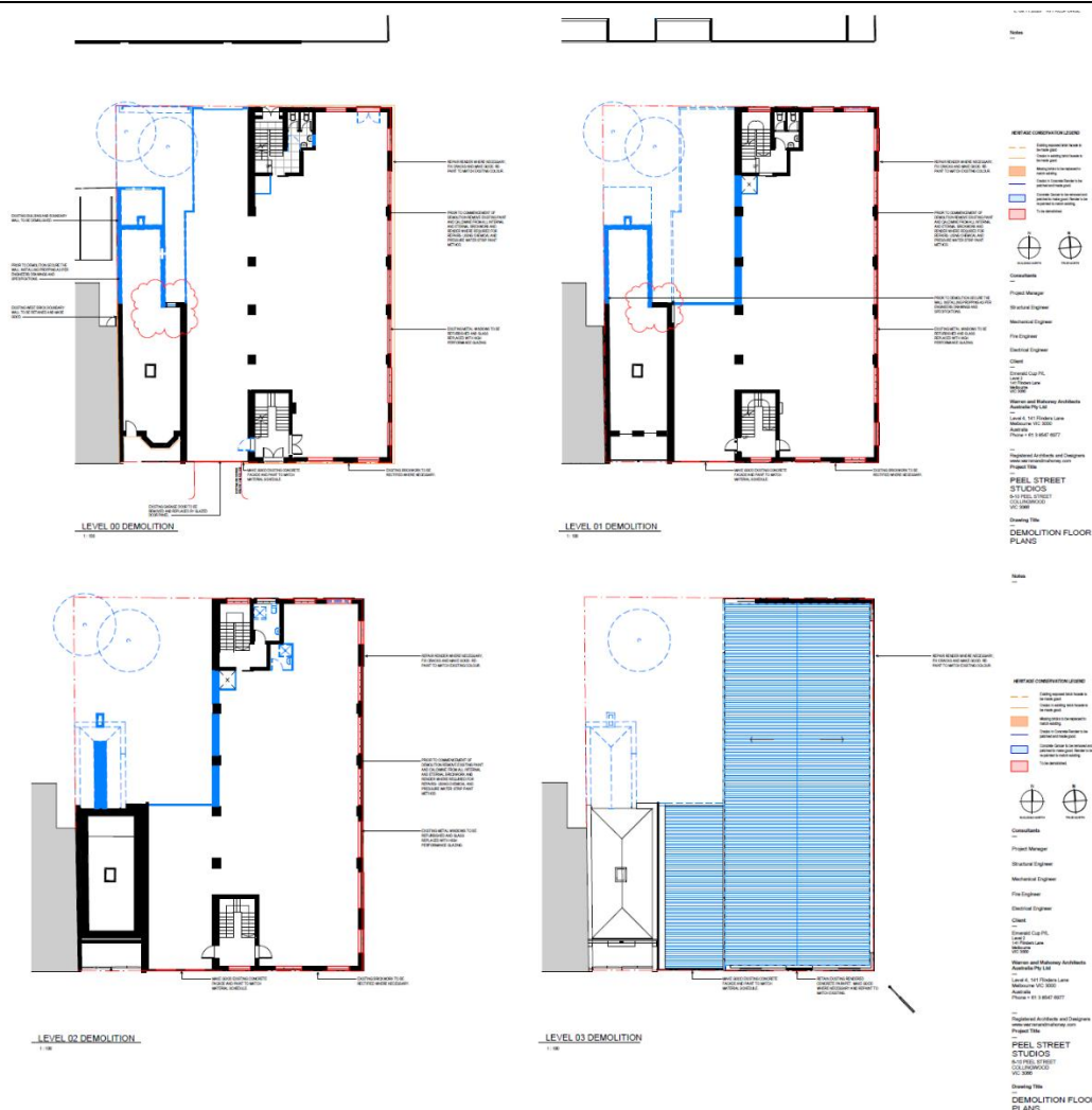
Figure: Demolition floor plans
