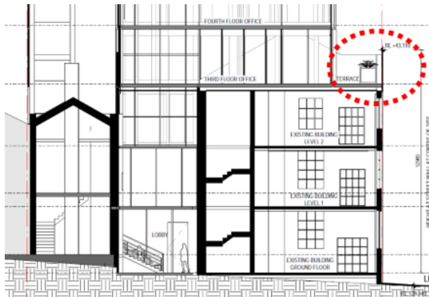
Figure: Extract from Section BB showing the relationship between the planters and parapet at Level 03
