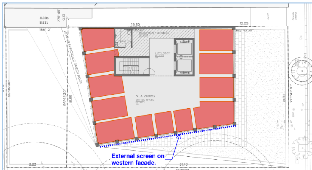
Figure 8: Level 6 daylight compliance areas shown in red.
