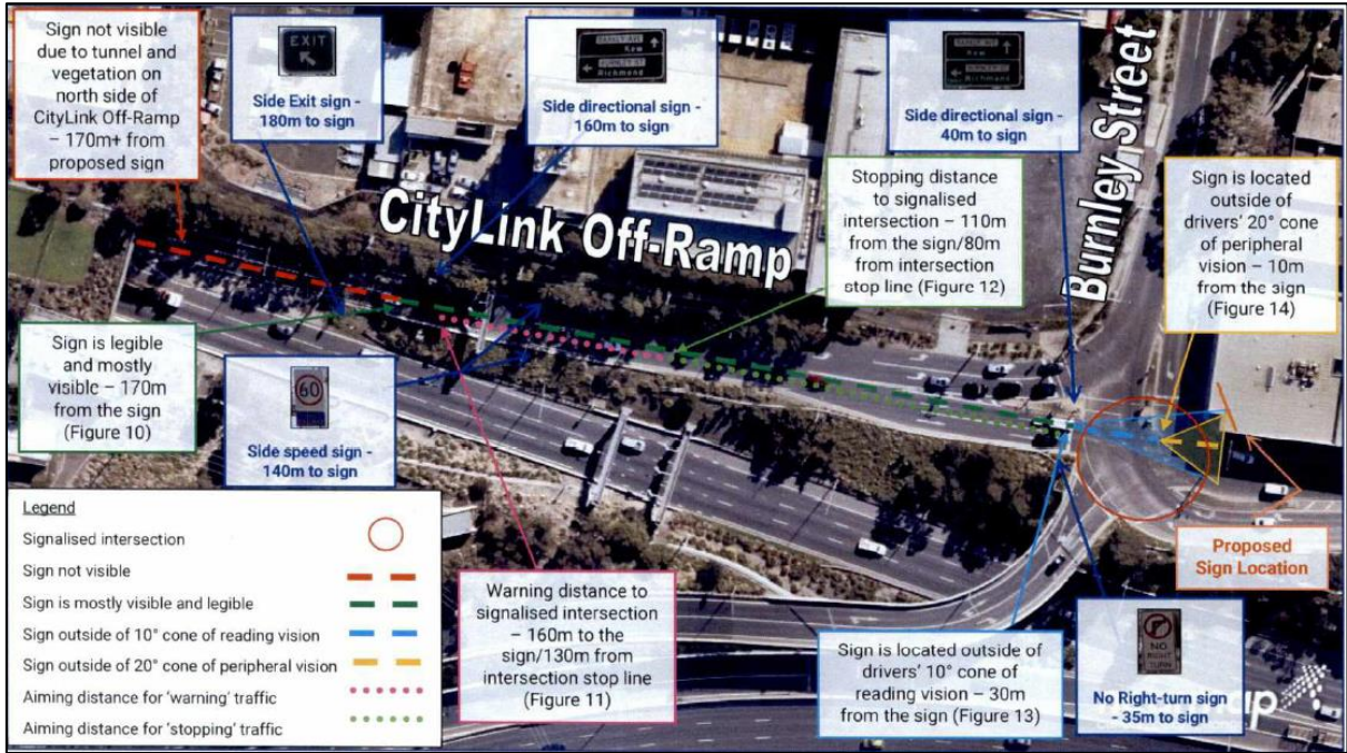
Figure 8 – CityLink off-ramp approach – Eastbound (Source: Traffic Group)
