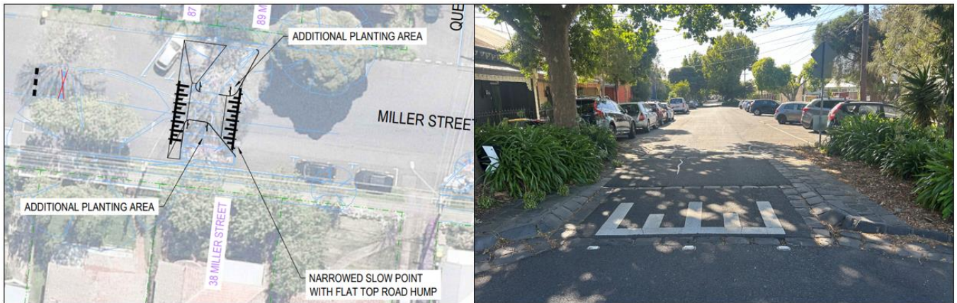
Figure 2: Proposed treatment design and example of similar type treatment on Noone Street, Clifton Hill
