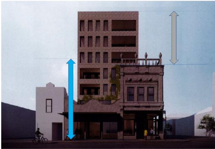
Figure 41: View 4 from the Urban Context Report, with dimensional arrows indicating that the visible height of the 2-storey heritage building is taller than the visible height of the new upper level form above/behind it. This is also important to achieving visual balance and recessive upper levels, and avoiding the upper levels being visually dominant over the heritage buildings.
