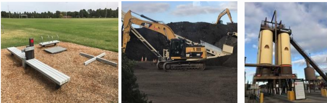
Recycled plastic park furniture Princes Park (left); Downer Somerton asphalt works (centre, right) using mix of asphalt, crushed glass (5-15%), plastics (0.7-1%), tyres (0.5%), toner (0.5%) for road making
