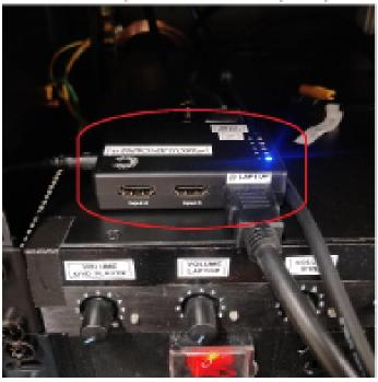
Make sure the light illuminated on the input selector box corresponds to the DVD Player. If it doesn't, you can change this by pushing the selector button until it does
