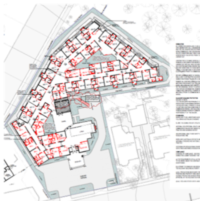
Picture 13 Proposed Internal Demolition
