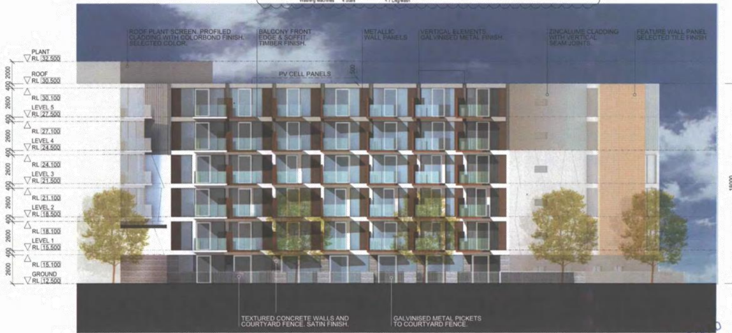
BLOCK D ELEVATION 02 (WEST END)
