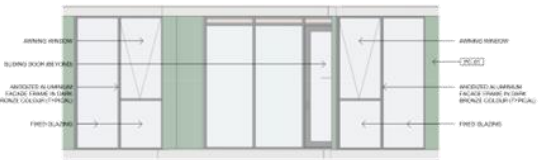
4 Elevation - East Operable Window 01 1:50
