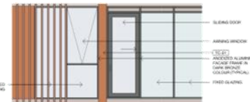
Elevation - South Operable Window 03 1:50
