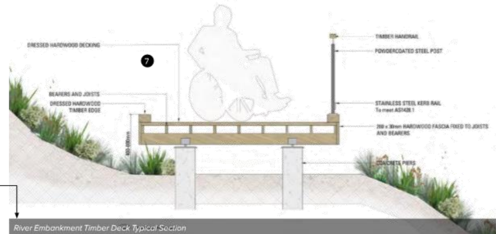
River Embankment Timber Deck Typical Section
