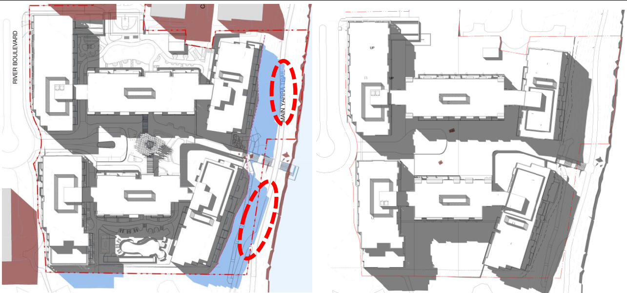
Images: 2pm September Equinox overshadowing diagrams of the original proposal (left) and amended proposal (right). Source: application documents.
