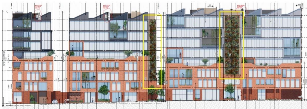
Figure 17. West elevation identifying vertical gardens.
