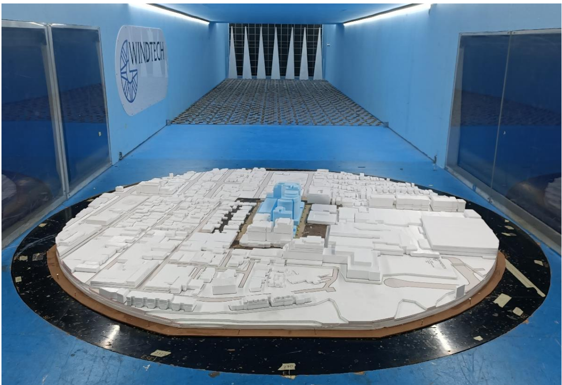
Figure 1c: Photograph of the Wind Tunnel Model (Proposed Site Conditions, view from the east)
