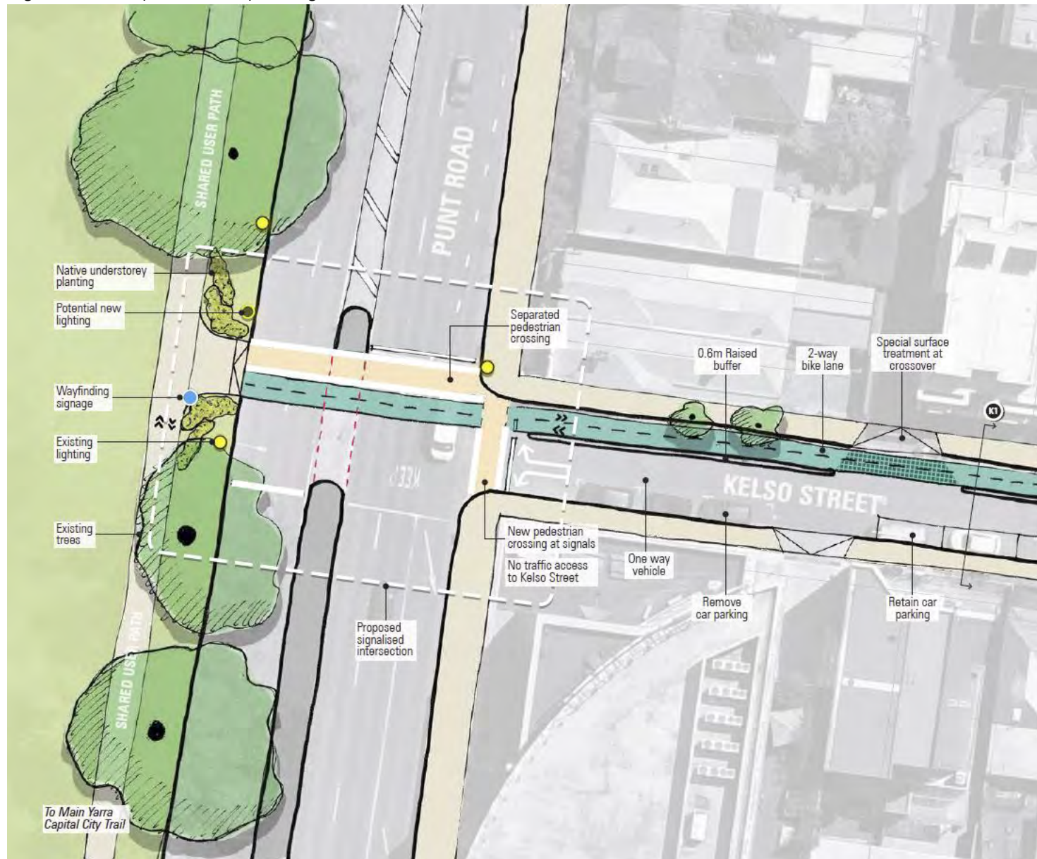
Figure 3 – Hotspot 1 concept design: Kelso Street - Punt Road intersection
