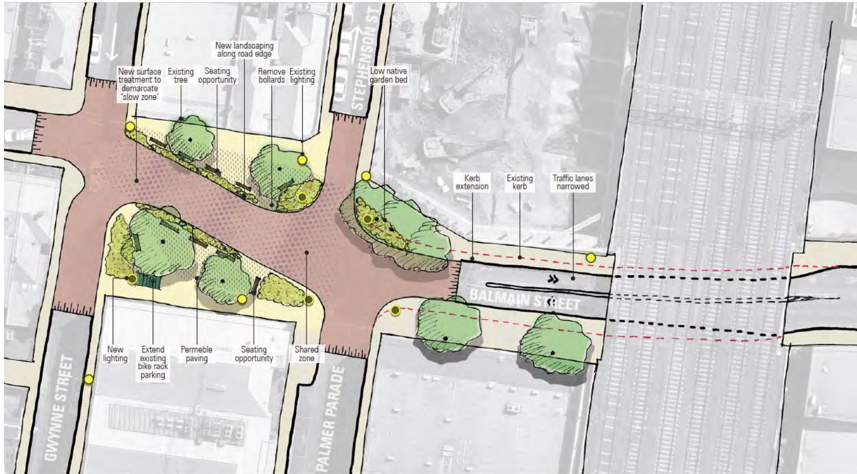
Figure 6 – Hotspot 4 concept design: Balmain Street west of underpass
