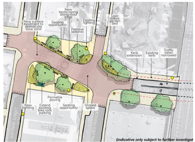
Figure 3.4 – Hotspot 4 - Balmain Street, west of the underpass
