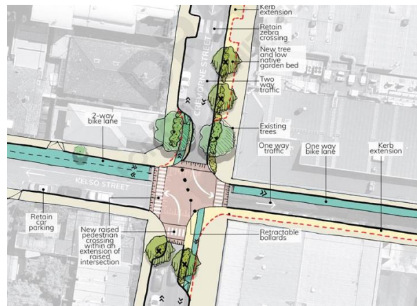
Figure 3.2 – Hotspot 2 - Cremorne Street and Kelso Street intersection
