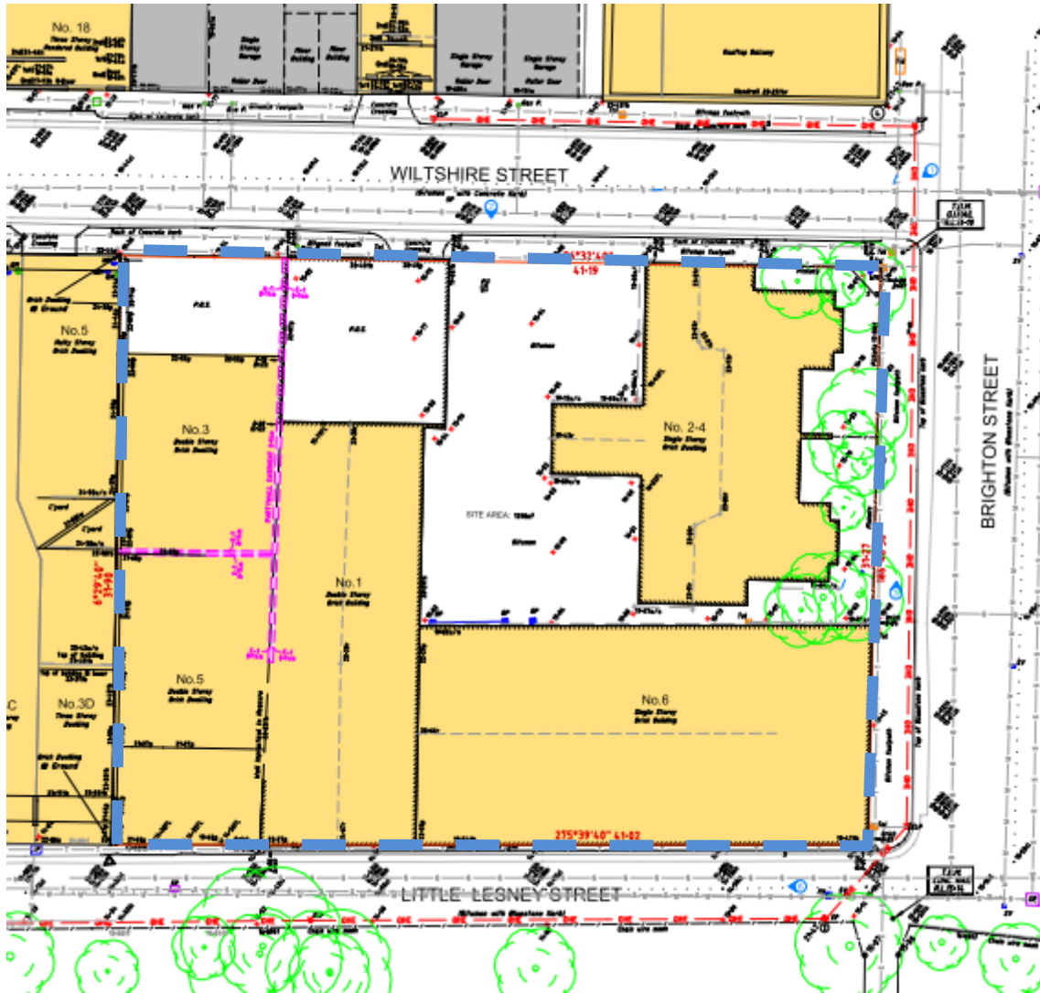
Image: Extract of survey plan of the Site (blue dashed outline) with existing easements shown in purple. Source: Advertised documents.
