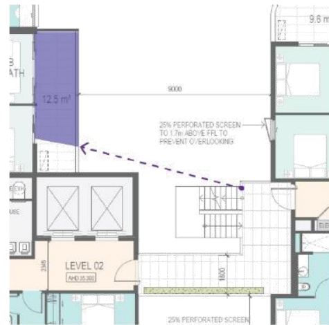
Extract of SD02_07, showing overlooking concerns
