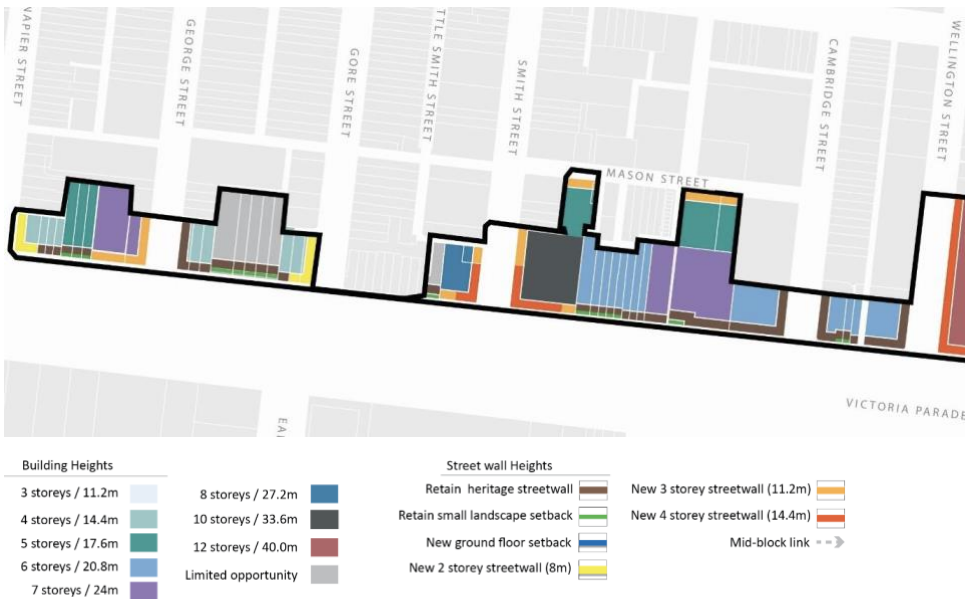
Figure 21. Extent of proposed DDO39 – Victoria Parade, west of Wellington Street, showing street wall and building heights. ('Map 1' from proposed DDO39)
