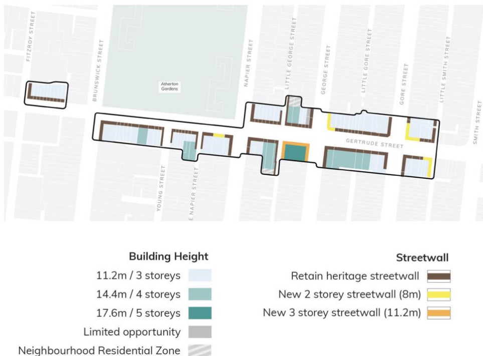
Figure 8. Extent of proposed DDO31 – Gertrude Street Shops, showing street wall and building heights. ('Map 1' from proposed DDO31)
