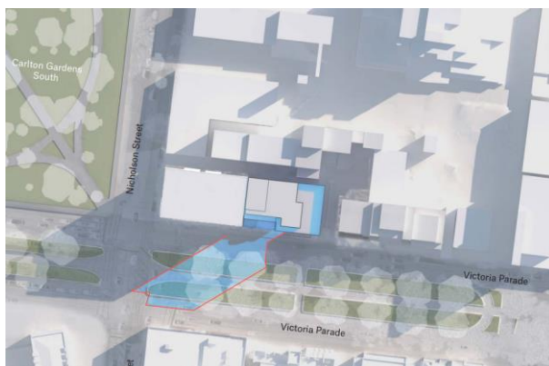
Figure 27 – Proposed 9am shadow (September 22 nd ) in blue (extract from p.70 of the Urban Context Report and Design Response).
