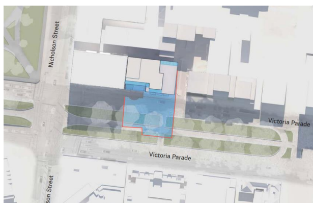
Figure 28 – Proposed 12pm shadow (September 22 nd ) in blue (extract from p.73 of the Urban Context Report and Design Response).
