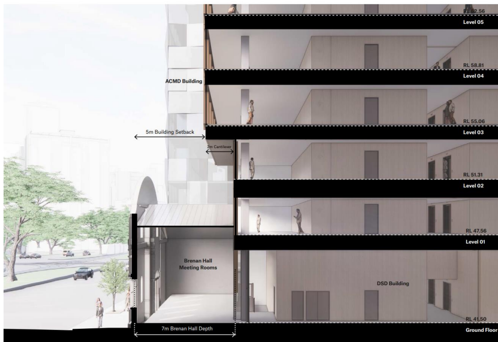
Figure 25 – Section showing cantilever of upper levels over the Brenan Hall extracted from p. 37 of the Urban Context Report and Design Response
