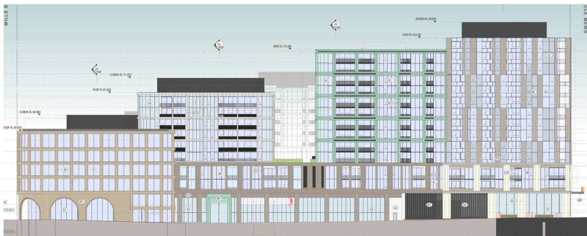
Figure 20: North Elevation, current proposal, reflecting a clearer transition in heights along the Heidelberg Road frontage (except from drawing TP2000 Rev.A).
