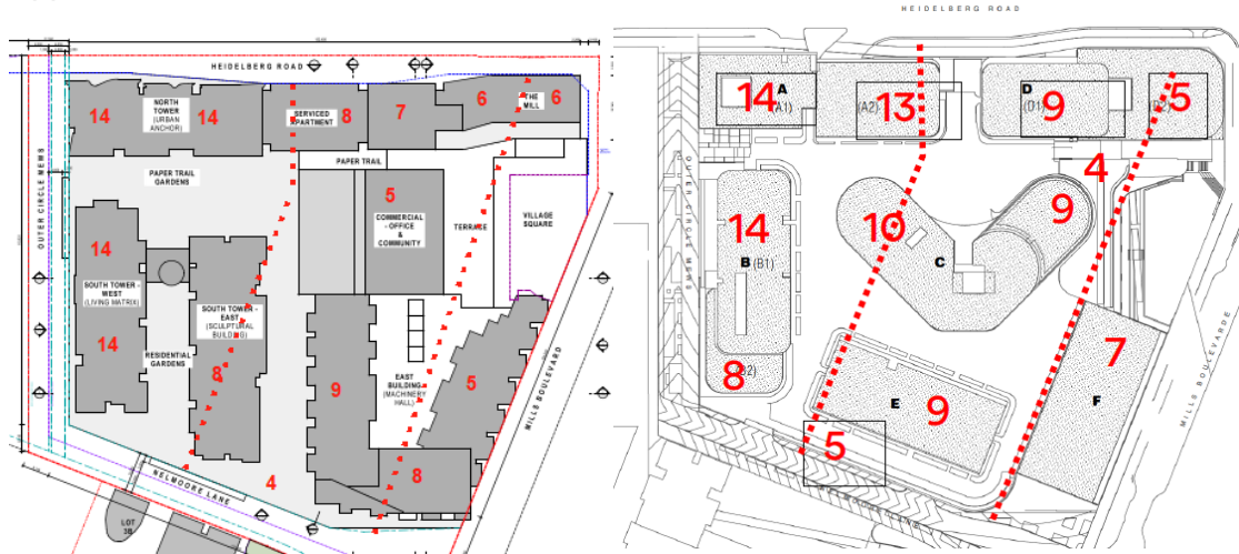
Figure 15: Left: previous site plan (with heights overlaid by officer), right: excerpt from external Urban Design advice of current proposal with heights overlaid.
