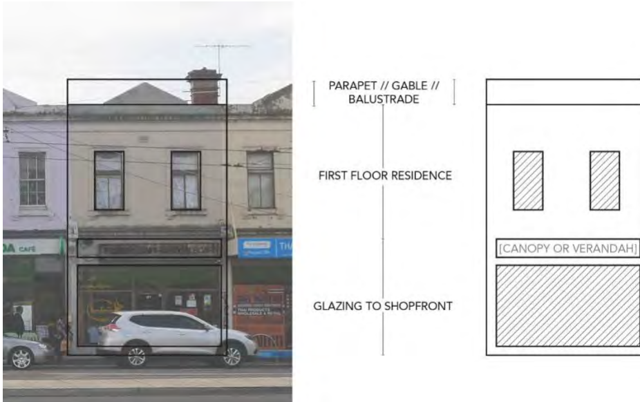
Figure 9 Diagram describing the typical ratio of solid surface area to glazing or apertures within heritage streetfronts. The proportion of glazing area across a streetfront elevation rarely exceeds 40% above the ground floor. (Address of example shown is 241 Victoria Street, which is located in Precinct 1).
