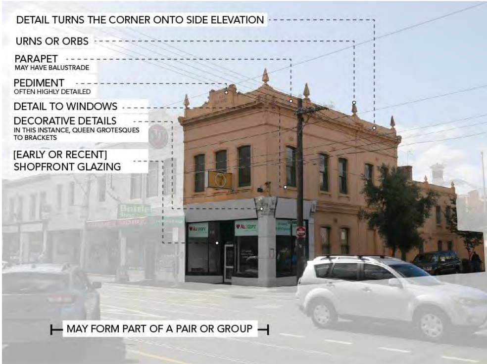
Figure 22. Shop/residence typology on a corner site with a return facade, showing typical features. This example is located within Precinct 3 at the northwest corner of Victoria Street and Park Street (address 277 Victoria Street).
