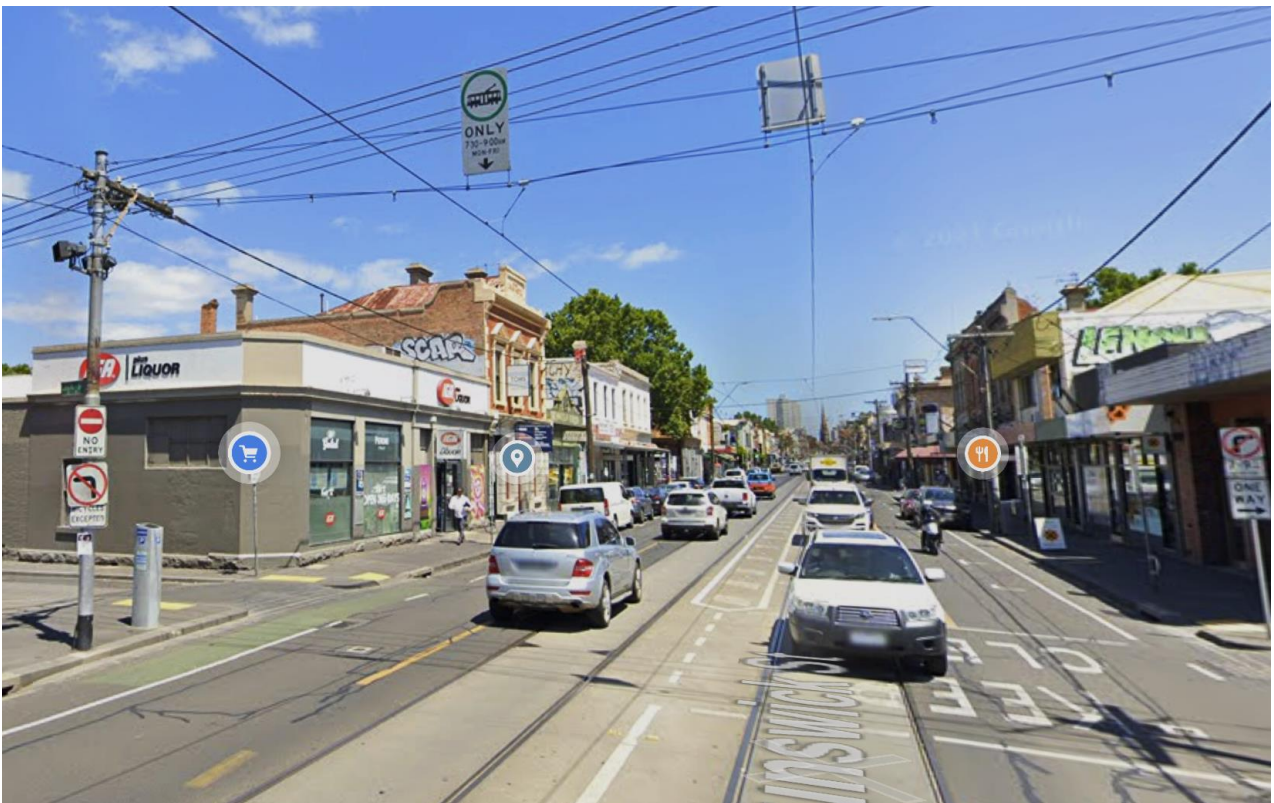
Figure 1 – The existing part time tram-lanes on Brunswick Street are linemarked with a simple yellow line and rely on drivers observing small overhead signs to see times of operation.
